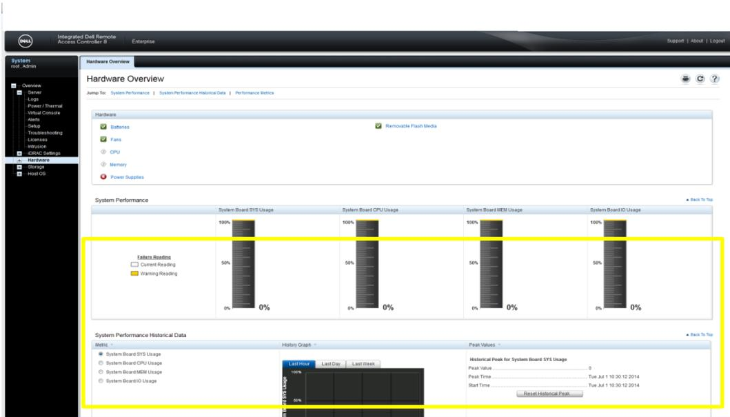
The **System Performance** table on **Hardware Overview** page, provides the current readings and warning threshold (upper non-critical) values for System, CPU, Memory and IO sensors.
