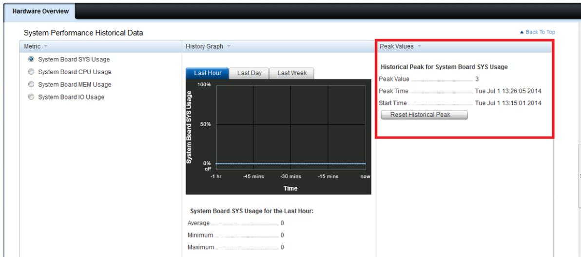
Click “**Reset Historical Peak**” button to reset the peak values of the sensors. This operation will reset the “Peak Value”, and update the “Peak Time” and “Start Time” of the corresponding sensor selected.
