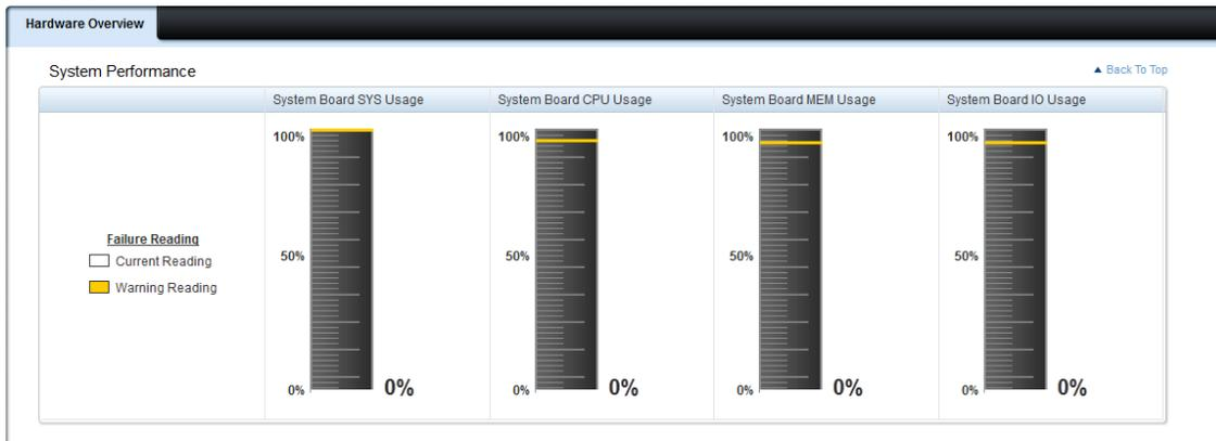
Traverse to **Performance Metrics** table on **Hardware Overview** page to configure the warning (upper non-critical) threshold values. User needs to enter the threshold values in the text box corresponding to the sensor and then click on **Apply** to configure the values.
