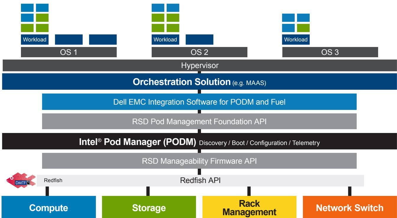
Intel® Pod Manager acts as a resource manager for disaggregated pools of hardware resources by communicating using standard Redfish APIs to hardware-aware software within the DSS 9000 called the Pooled System Management Engine (PSME). PODM provides configuration management of the pools of compute, storage and networking resources to administrators and applications through a vendor-agnostic orchestration (RESTful) API. (See Figure 2).
