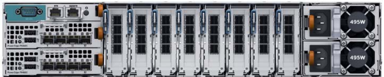
Figure 3 Dell PowerEdge FX2s (back) with two PowerEdge FN410S IOMs installed
