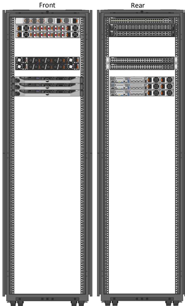
Figure 118 Rack containing management or edge cluster and spine switches
