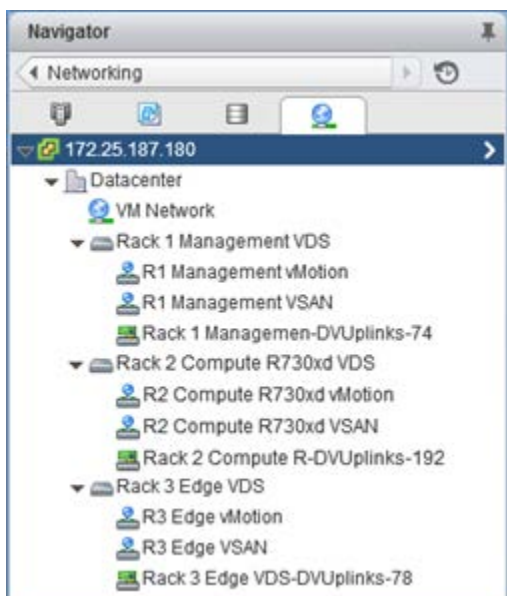
Figure 32 Distributed switches with vMotion and VSAN port groups created
