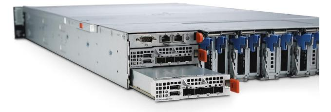
Figure 5 FX2 chassis with FN IOM (FN410S shown)
