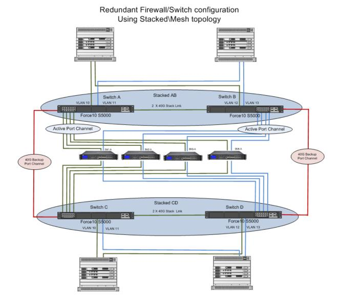
In the above design, security layer links are shown in a single active port-channel with dual links to each firewall; however, they can be configured as needed to support scaling or additional VLAN's for ingress/egress. The reference design also includes a bypass port-channel which serves to back-up the active links. If the security layer fails or must be taken out of service, it can be quickly and easily bypassed using this method.
