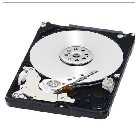
Figure 1: Hard disk drive with cover removed, showing spindle, platters and read/write arm
