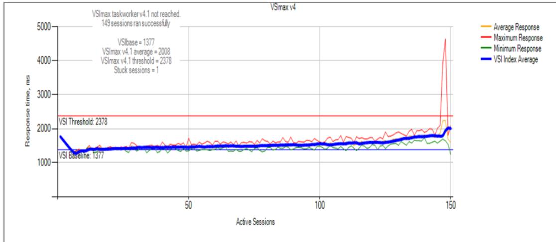
The Task Worker workload didn't quite reach the 85% mark but VMs configured with only one vCPU tend to load the CPU less. The E5-2660 v4 processor was used for the V470/V470F-B5 testing.
