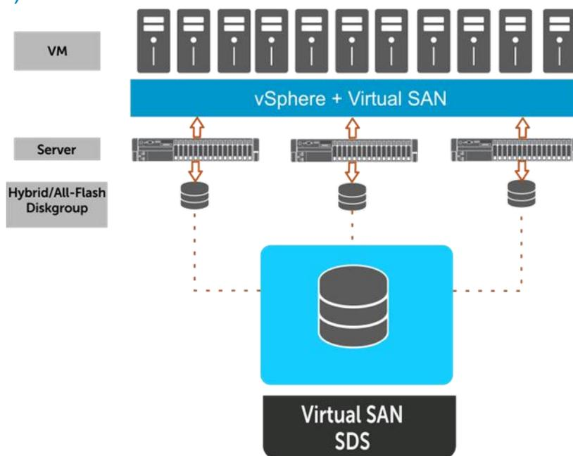
VMware vSAN is software-defined storage solution fully integrated into vSphere. Once enabled on a cluster, all the flash or magnetic hard disks present in the hosts are pooled together to create a shared data store that will be accessible by all hosts in the VMware vSAN cluster. Virtual machines can then be created and a storage policy can be assigned to them. The storage policy will dictate availability / performance and sizing.
