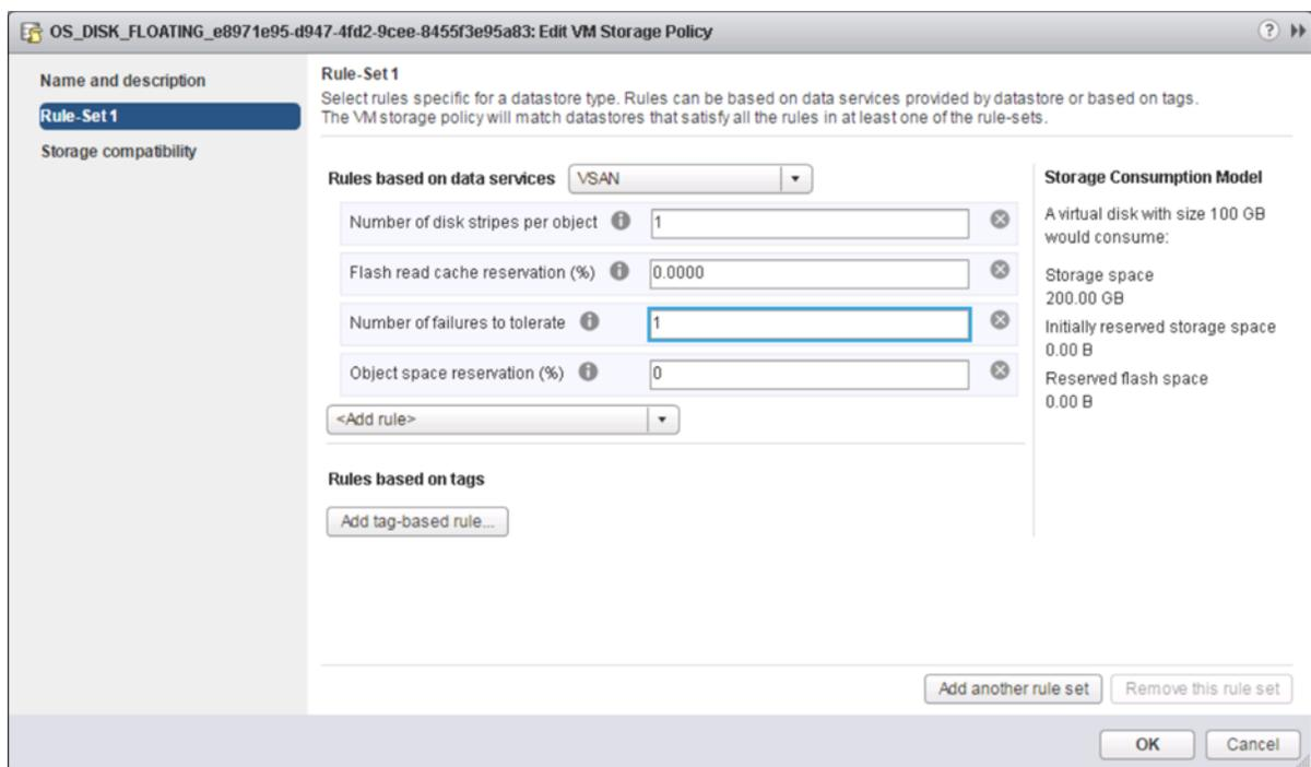
The recommended configuration by VMware for a VMware vSAN Cluster with FTT=1 and RAID 1 is four nodes and this ensures that the virtual machines are fully protected during operational & maintenance activities. This configuration can also survive another failure even when there is a host already in maintenance mode.
