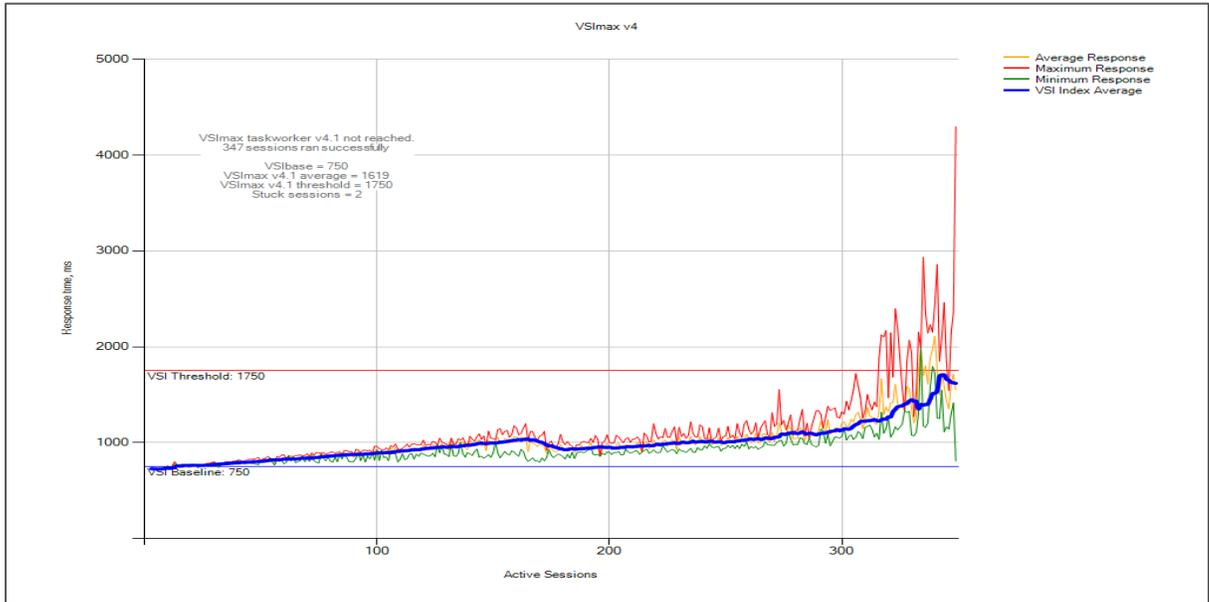
The host CPU was pushed to a 92% steady state average during this test run and the two sampled RDSH VMs to approximately 80% each. The data suggests that 350 Task Worker users are at the upper end of the capabilities of this config.
