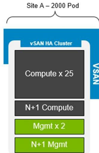
The recommendation from VMware is not to exceed 2,000 VM's/Sessions per Block and once we have more than 2000 VM's we would then split the management and compute into separate vSAN Clusters. The example below shows a scale out of a 10,000 user Horizon vSAN Pod with 2000 user blocks, each block contains its own Virtual Center, Horizon connection & composer servers.
