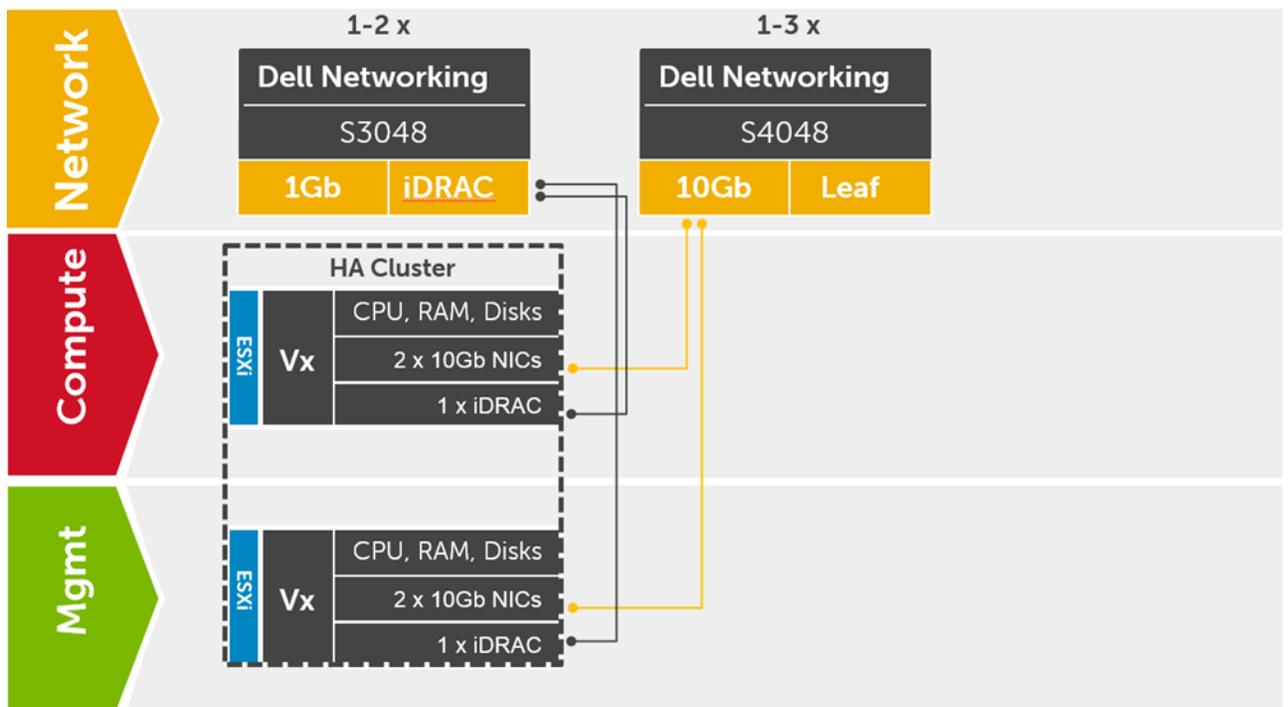
The following figure shows a design of a scale-out Leaf-Spine network architecture that provides 20 GB active throughput from each node to its Leaf and scalable 80 GB active throughput from each Leaf to Spine switch providing scale from 3 VxRail nodes to 64+ without any impact to available bandwidth:
