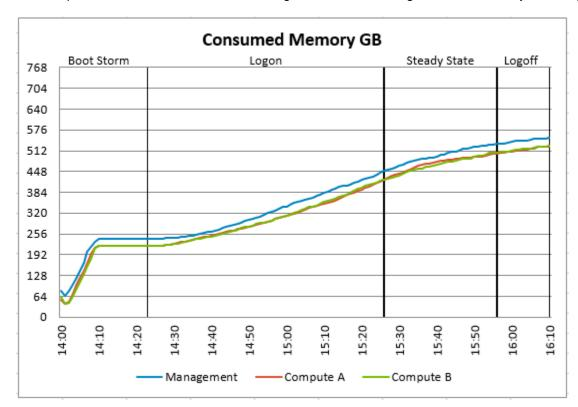
Active memory usage reached a maximum of 416 GB on the Compute B host during the Boot Storm, and the average Steady State usage for all hosts was 154 GB. Each desktop used 0.96 GB of active memory after deducting for CVM and management VM usage. The CVM used its full 32GB of active memory throughout the test run.
