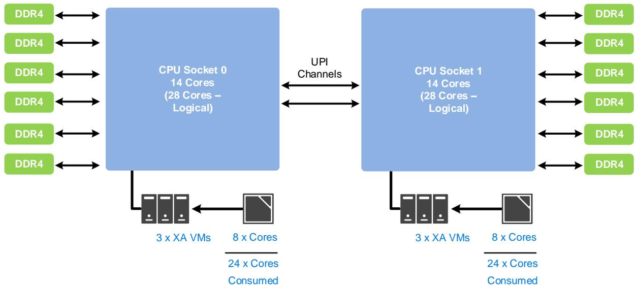
**NOTE:** To ensure no NUMA spanning, remove the checkmark for “Allow virtual machines to span physical NUMA nodes” in the Hyper-V settings of the compute host(s). Also ensure “Maximum NUMA nodes allowed on a socket” is set to a value of 1. This setting is found under Processor > NUMA for each RDSH VM.
