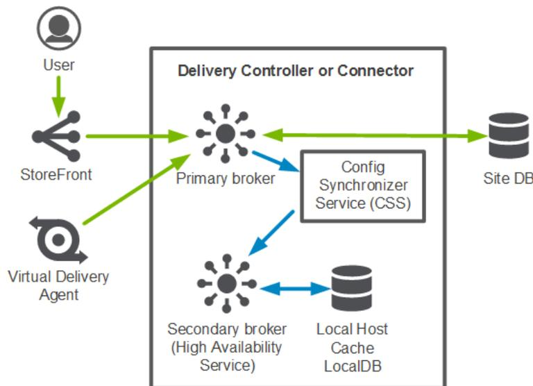
The diagram below illustrates changes in communication when the principal broker is unable to connect to the Site database.
