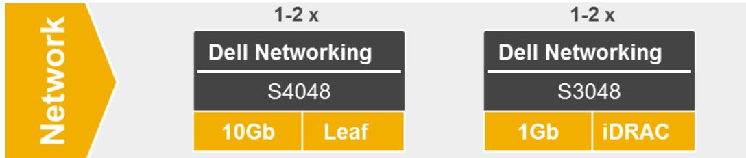
Each Dell EMC S2D Ready Node is equipped with dual port RDMA network adapters for host and storage traffic. Although the solution can function with a single switch, Dell EMC highly recommends redundant top-of-rack S4048 switches. Each RDMA port is connected to a different S4048 switch in this scenario.
