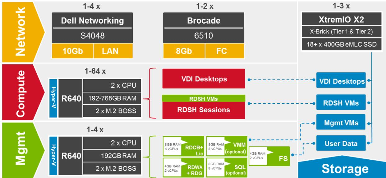
**NOTE:** Minimum disk configuration per XtremIO X2 X-Brick is 18 x 400GB SSDs which is sufficient for up to 3500 VDI users. Additional disks may be required if increased capacity is needed for larger personal disk sizes and if user data is also stored on the array.
