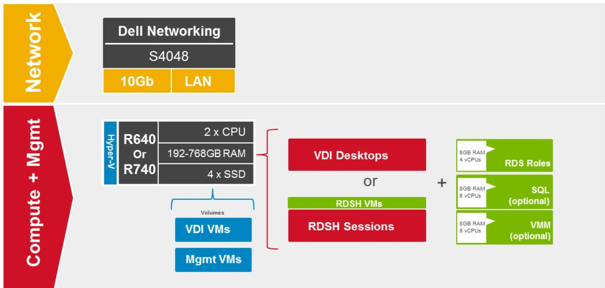
**NOTE:** This configuration can support up to 150 users based on the Task Worker workload.
