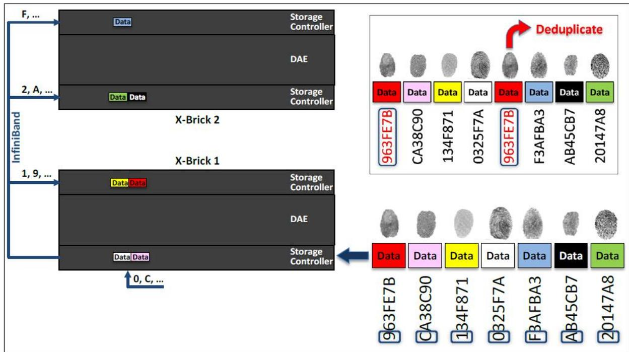
Using the same unique fingerprints, XtremIO is equipped with exceptional always-on in-line data deduplication abilities, which highly benefits virtualized environments. Together with its data compression and thin provisioning capabilities (both also in-line and always-on), it achieves incomparable data reduction rates. The figure below demonstrates capacity savings with in-line deduplication and compression prior to the data being written.
