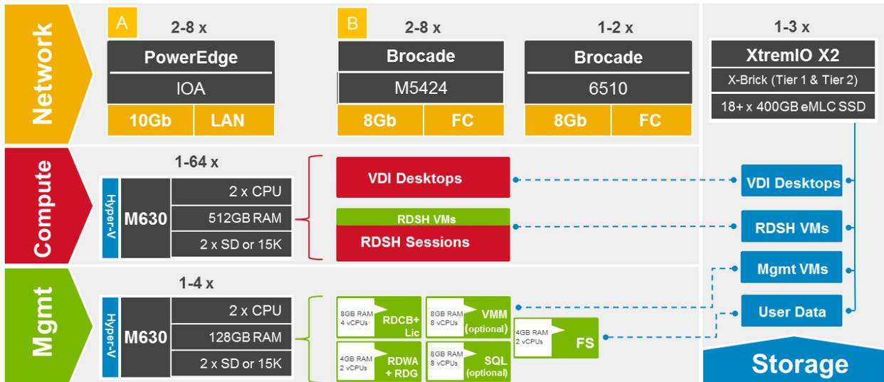
**NOTE:** Minimum disk configuration per XtremIO X2 X-Brick is 18 x 400GB SSDs which is sufficient for up to 3500 VDI users. Additional disks may be required if increased capacity is needed for larger personal disk sizes and if user data is also stored on the array.
