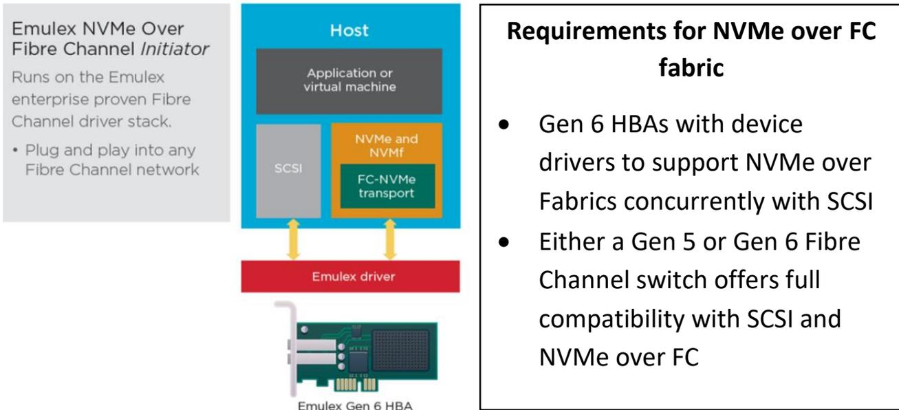
Figure 2: Dell EMC branded NVMe-over Fibre Channel Adapters plug and play into any FC network.
