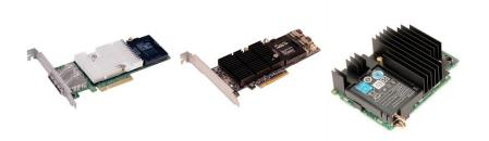
The DellEMC PERC offers iDRAC sideband management integration which allows agentless management of the RAID controllers. This enables configuration, monitoring and alerting of the PERC and does not require any additional software installed. It also allows remote management of the PERC.
