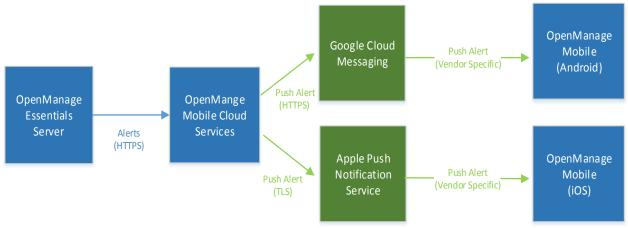
Figure 1 Alert Push Notification Security
