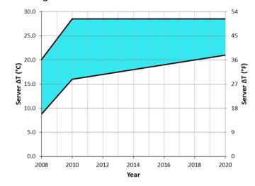
Source: Fig. "Server ∆t projection at 25°C (77°F) server inlet temperature"; *IT Equipment Design Impact on Data Center Solutions*; ASHRAE 2016
