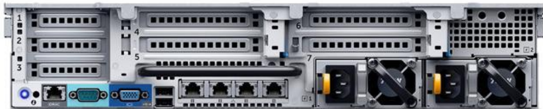
Figure 4 – Rear view of an R730 rackmount server with dual Power Supply Units (PSU)
