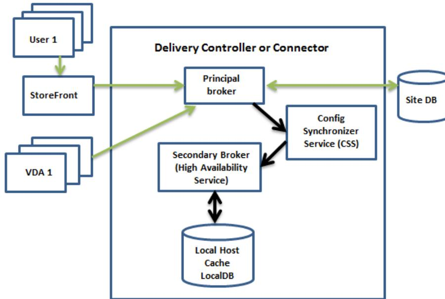
The following diagram illustrates changes in communication when the principal broker is unable to connect to the Site database.
