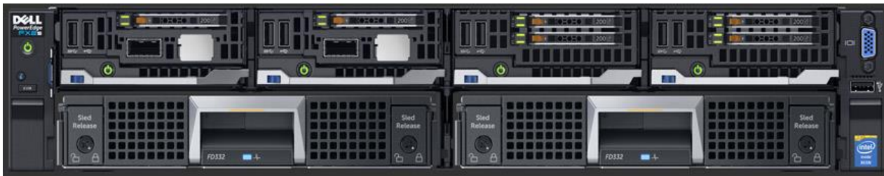
Figure 1 Dell PowerEdge FX2s (front) with four PowerEdge FC430 servers and two FD332 storage sleds
