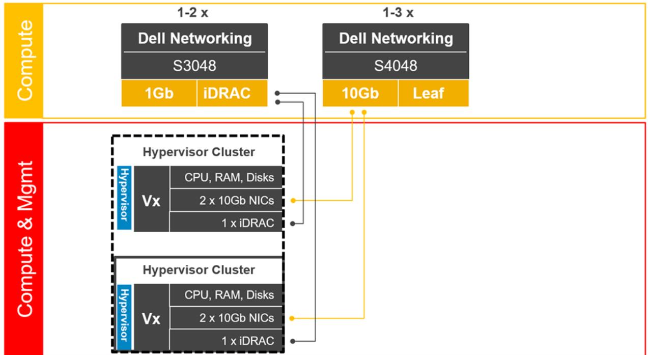
The following figure shows a design of a scale-out Leaf-Spine network architecture that provides 20 GB active throughput from each node to its Leaf and scalable 80 GB active throughput from each Leaf to Spine switch providing scale from 3 VxRail Appliance nodes to 64 without any impact to available bandwidth:
