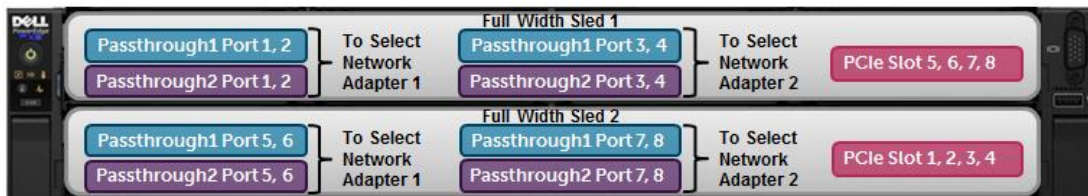
Figure 11 Front layout of FX Chassis with FM120x4 sleds
