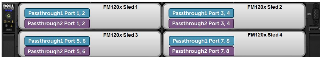
Figure 11 Front layout of FX Chassis with FM120x4 sleds
