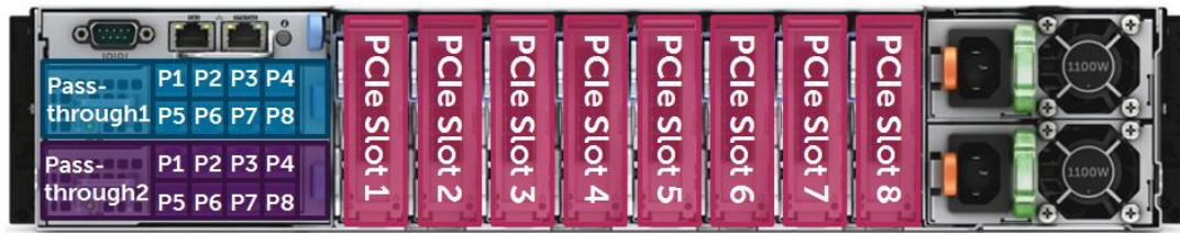
Figure 8 Front layout of FX Chassis with Quarter-width sleds
