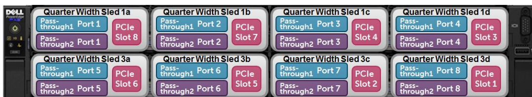
Figure 8 Front layout of FX Chassis with Quarter-width sleds
