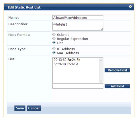
Figure 6. MAC Authentication ClearPass - Create Static Host List
