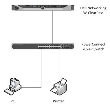
The figure above shows the setup used for this document. The printer is used for the MAC Authentication example configuration, while the PC is used for the OnGuard heath posture example configuration.
