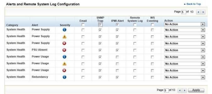
Figure 5. Configuring SNMP Trap alerts
