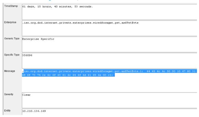
In the trap details, note the contents of the **Specific Type** field, which are 356096 in this sample. Match 356096 to the DcAsfSrv.mib file, which has the following information for a chassis intrusion event:
