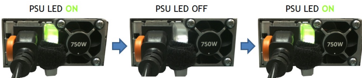
Figure 2. The PSU LED flashes on and off at a rate of 1Hz to indicate a PSU mismatch
