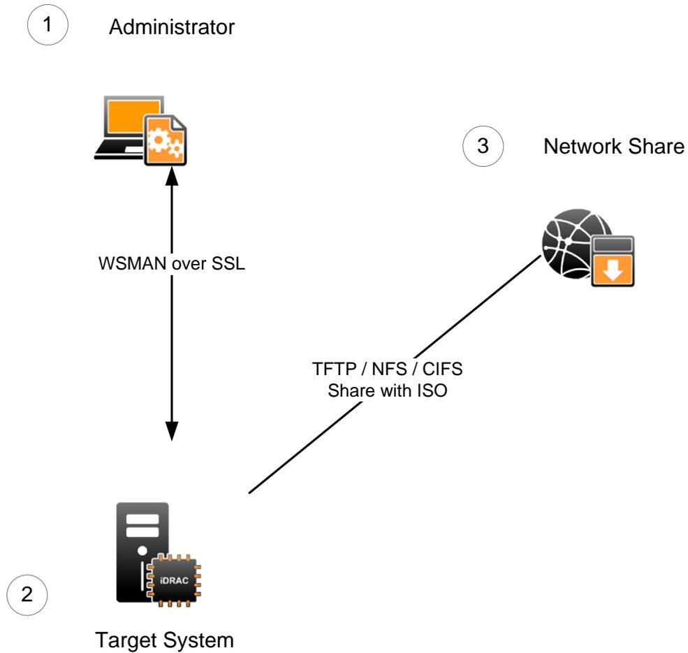
Figure 1 shows the pictorial view of the environment. It starts with administrator (1) running scripts to send WSMAN commands through an SSL connection. The target system (2) is a Dell PowerEdge 11G or later server equipped with iDRAC service processor. The network share (3) is used to attach the ISO image to the target iDRAC's host. The iDRAC's host will boot to the emulated USB holding the ISO image.
