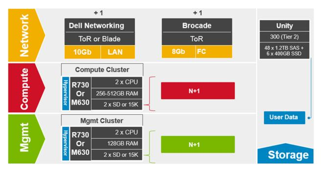
The HA options provide redundancy for all critical components in the stack while improving the performance and efficiency of the solution as a whole.
