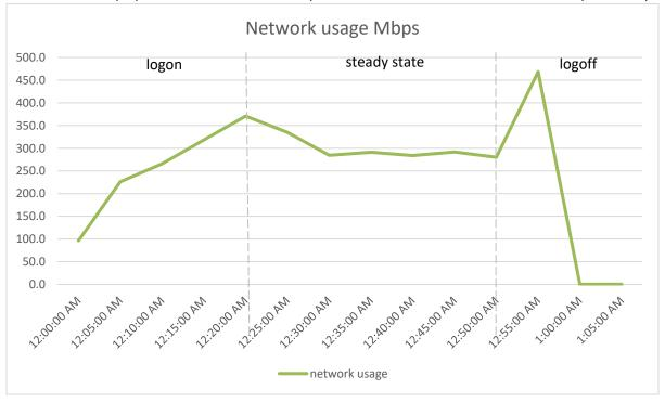
Network usage of the Power worker workload tests showing heavier usage than other two workloads. Peaked at around 4.5 Mbps per user, and under 500Mbps on the host. It is still well under the 1Gbps NIC capacity.
