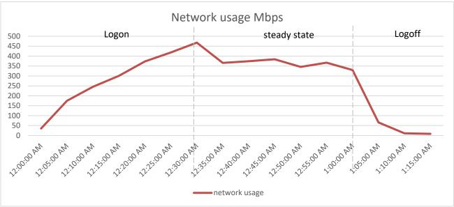
Network bandwidth is not an issue on this test run with a steady state peak of approximately 2Mbps per user which was just over 400Mbps overall on the host.
