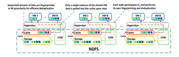
Nutanix Shadow Clones delivers distributed localized caching of virtual disks performance in multi-reader scenarios, such as desktop virtualization using VMware Horizon or RDSH. With Shadow Clones, the CVM
