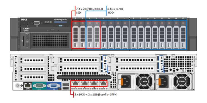
Important to note that this platform must be configured using CPUs with a max TDP of 120w and requires 1100w PSUs.
