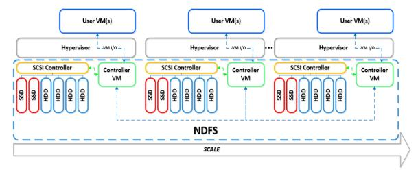
NDFS understand the concept of a virtual machine and provides advanced data management features. It brings data closer to virtual machines by storing the data locally on the system, resulting in higher performance at a lower cost. Nutanix platforms can horizontally scale from as few as three nodes to a large number of nodes, enabling organizations to scale their infrastructure as their needs grow.
