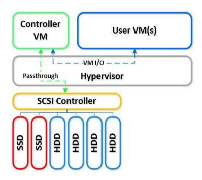
In addition, local storage from all nodes is virtualized into a unified pool by the Nutanix Distributed File System (NDFS). In effect, NDFS acts like an advanced NAS that uses local SSDs and disks from all nodes to
