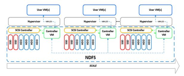
NDFS understand the concept of a virtual machine and provides advanced data management features. It brings data closer to virtual machines by storing the data locally on the system, resulting in higher performance at a lower cost. Nutanix platforms can horizontally scale from as few as three nodes to a large number of nodes, enabling organizations to scale their infrastructure as their needs grow.
