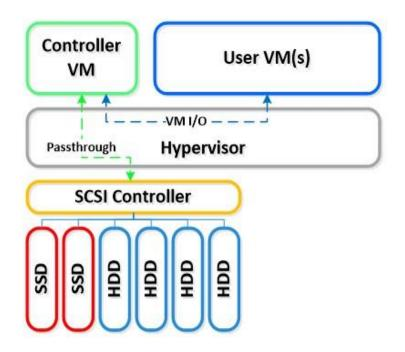
In addition, local storage from all nodes is virtualized into a unified pool by the Nutanix Distributed File System (NDFS). In effect, NDFS acts like an advanced NAS that uses local SSDs and disks from all nodes to store virtual machine data. Virtual machines running on the cluster write data to NDFS as if they were writing to shared storage.
