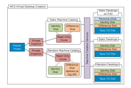
While traditionally used for small to medium sized XenDesktop deployments, MCS can bring along with it some substantial Tier 1 storage cost savings because of the snapshot/identity/difference disk methodology. The Tier 1 disk space requirements of the identity and difference disks when layered on top of a master image snapshot, is far less than that of a dedicated desktop architecture.
