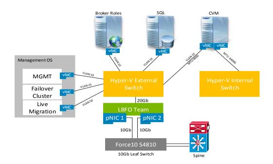
The NIC team for the Hyper-V switch is configured as switch independent, Dynamic for the load balancing mode with all adapters set to active. This team is used exclusively by Hyper-V.
