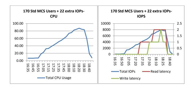
The login script launched an automated Iometer workload in each VDI session to generate extra IOPs within the session. This generated sustained IOPs of approximately 8000. As can be seen from the graphs above the latency of the local tier 1 storage on the SSD volumes did not rise above 2 milliseconds which is well within the bounds that are considered appropriate for VDI performance (i.e. < 20ms)
