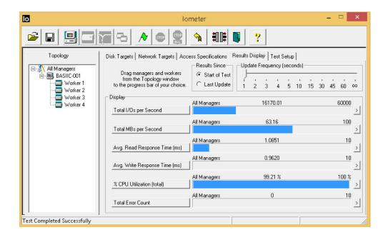
It can be seen that at 16000 IOPs with 80% write the latency remains at approx. 1 millisecond. While IOMETER test scenarios are very subjective and it is arguable whether the test specification used above truly represents a VDI workload, it does represent a reasonable approximation and the result of 16000 IOPs available on the SSD volume does indicate that it is possible for the solution to support much more IO intensive workloads as indicated in the following graph:
