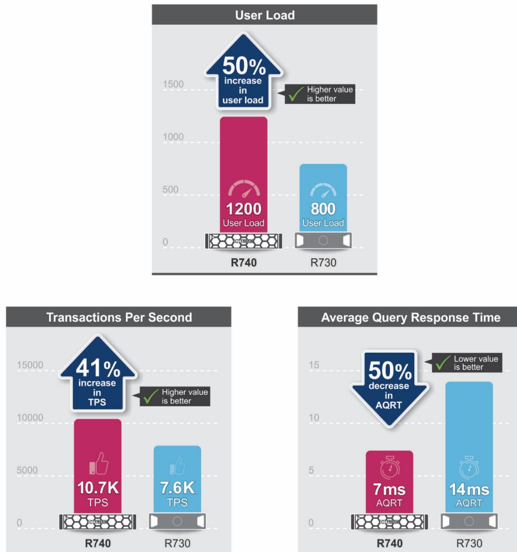
Figure 4 Performance comparison – SQL Server 2016 on PowerEdge R740 and PowerEdge R730
