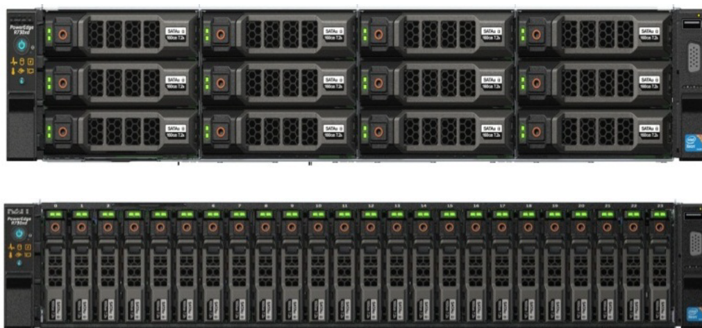
Figure 2: Dell EMC PowerEdge R730xd Servers - 2.5" and 3.5" Chassis Options
