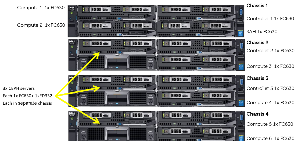
Figure 1: Dell EMC PowerEdge FX2 Chassis Layout
