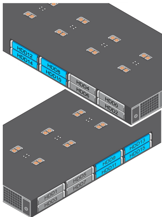
Figure 5: Storage Sled Dell EMC PowerEdge FD332 Drive Layout
