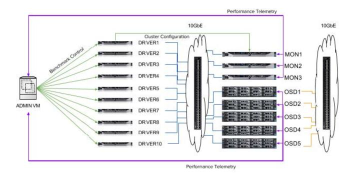
The utility is installed on Monitor Node 3. From there, it communicates with various servers in different capacities via *pdsh* as follows:
