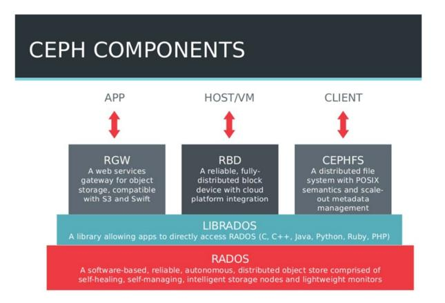
Writing and reading data in a Ceph storage cluster is accomplished by using the Ceph client architecture. Ceph clients differ from competitive offerings in how they present data storage interfaces. A range of access methods are supported, including:
