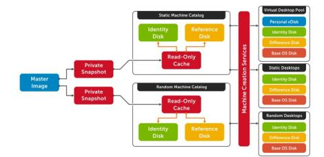
While traditionally used for small to medium sized XenDesktop deployments, MCS can bring along with it some substantial Tier 1 storage cost savings because of the snapshot/identity/difference disk
