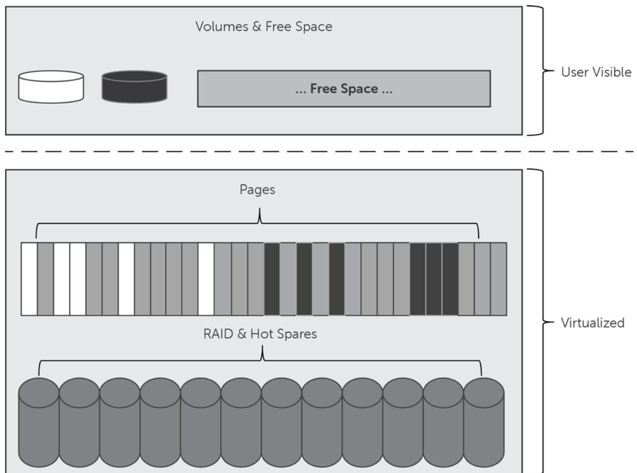
**Figure 5 - How EqualLogic storage is virtualized**
